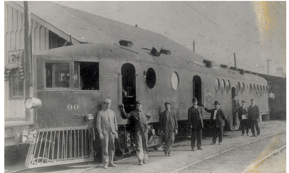
1918 Scooter to Munden Point - Ran from Norfolk to Munden Point 1910 to 1929. Initially gasoline and became electric in 1923. Courtesy of The Virginia Beach Public Library, Edgar T. Brown Collection.
