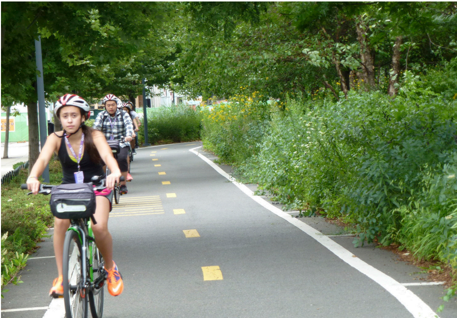
Figure 42: Centerline and edgeline marking
